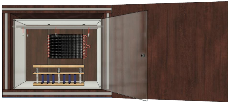
Fig. 1.1: Acrylic Hinged, Front-Load Cell Test Chamber Drawing – Front view
